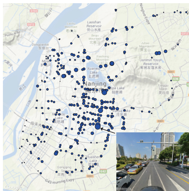
Fig. 2. Locations of all transportation cells in Nanjing. Each circle represents one cell, with its area being proportional to flow volume on Dec. 1st, 2012. A picture of the busiest cell is shown in the inset.
