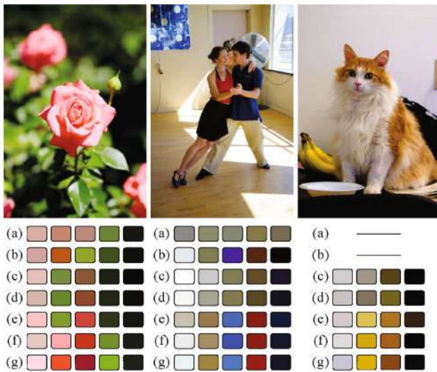
Fig. 14 Examples of images and their associated color palettes generated by O’Donovan et al. [15] (a), Lin and Hanrahan [18] (b), Shapira et al. [36] (c), k -means (d), Chang et al. [20] (e), Zhang et al. [24], and our method (g). Our results provide a more discriminable palette. For example, in the middle photo, our method chooses a brighter blue, which is more separable from the dark blue. Testing images and palettes for other methods are taken from Zhang et al. [24].
