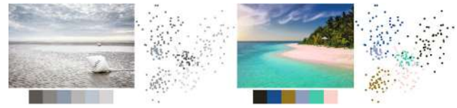
Fig. 21 Left: an undesirable color mapping that fails to distinguish classes from each other. Right: a good one. The respective class separation scores are 11,555 and 19,477. The quality of our generated color mappings depends on the reference images.
